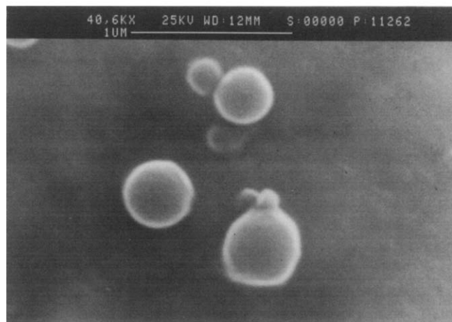
Figure 4 SEM micrograph of polystyrene-containing DODAB vesicle (original magnification 40 600 ×; bar indicates 1 μm)
